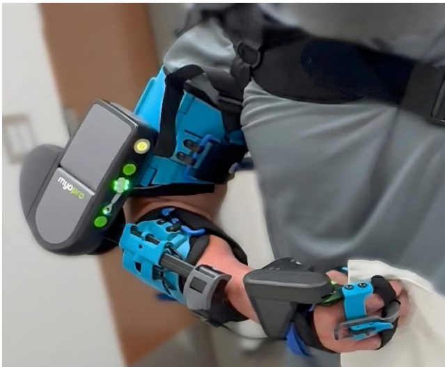
Figure 1: The MyoPro®, a commercial myoelectric orthosis manufactured by Myomo, Inc. The device assists hemiparetic patients with hand and elbow function. Each device is custom fabricated to the patient. Two motors are controlled by two pairs of surface electromyography electrodes. The elbow motor controls elbow flexion or extension. The hand motor controls opening and closing the hand. The device is battery powered, and can be used in therapy, at home, or out in the community.
